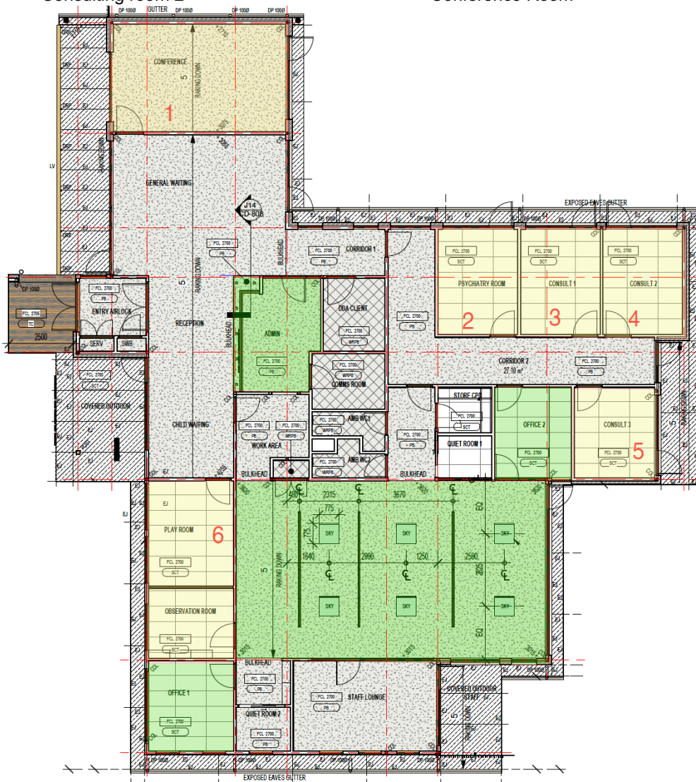
Figure 1 Proposed internal layout including Consulting Rooms Numbered in red (6 total) shaded in yellow. Staff areas are shaded in green.
