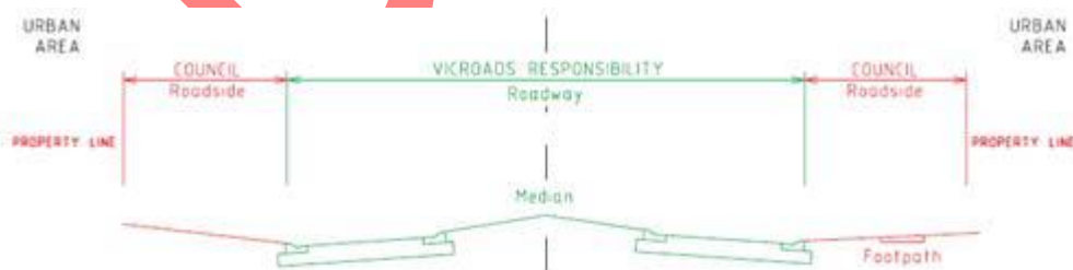
Figure 3 – Demarcation Arrangements for Typical Rural Arterial Roads
