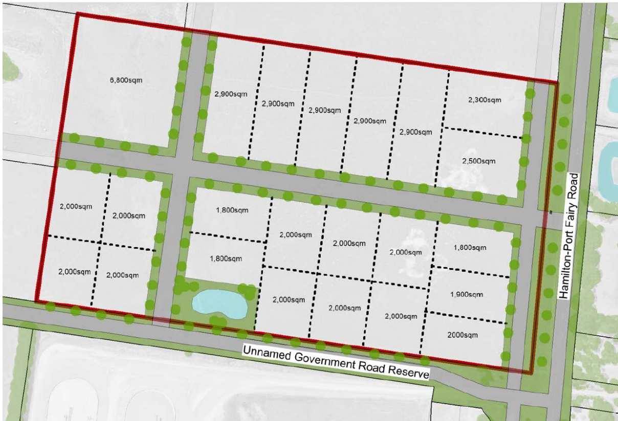
Drawing 1: The preliminary concept plan shows the one access road to subdivisions from Hamilton-Port Fairy Road.
