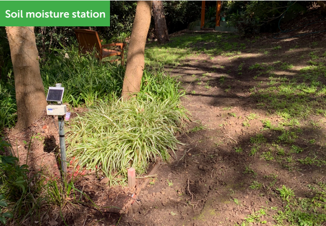
Soil moisture probe and station installation
